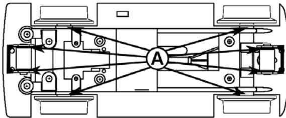
Please refer to the figure above. The wheels and roller pickups require electrical flow, therefore we recommend using Bachmann E-Z Lube® #99981 Conductive Contact Lube on all points **Marked A**. **Never use any Teflon® based oil on these areas because this type oil has insulating properties.**
