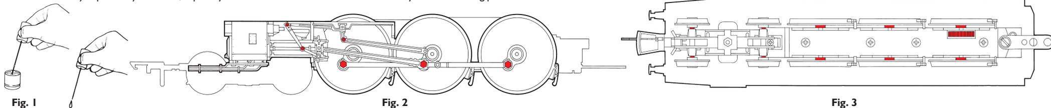
Apply one drop of oil to each of the valve gear and connecting rod pivot points indicated in red in Fig.2, on both sides of the locomotive.
