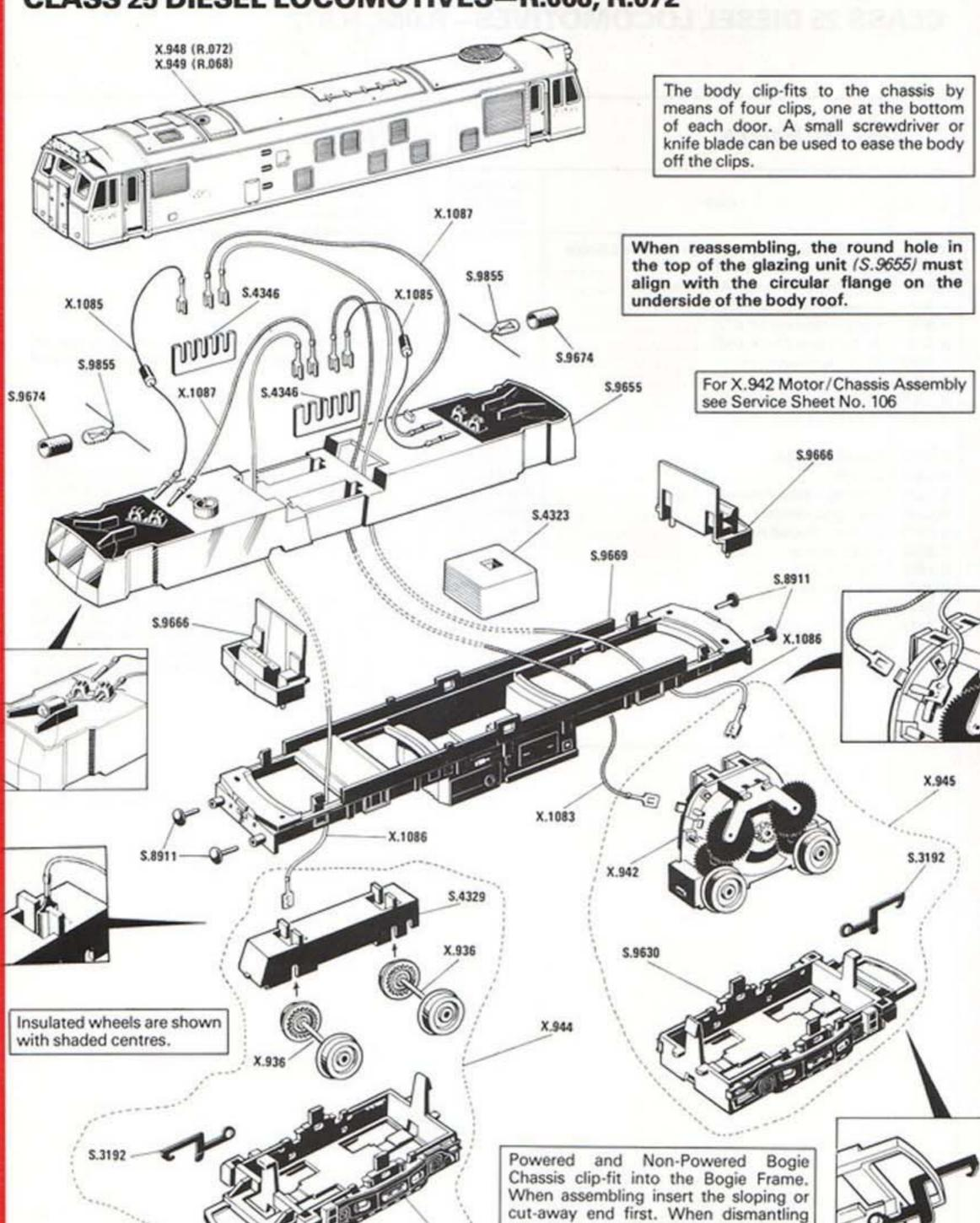
When assembling the non-powered bogie ensure that the insulated wheels (shaded centres) are on the correct side.
